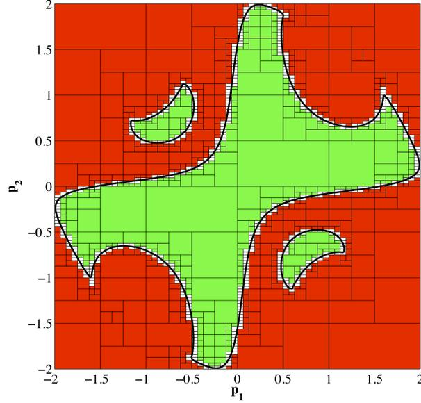
Figure 2:  $\mathcal{F}^{\text{sub}}$  (red) and  $\mathcal{S}^{\text{sub}}$  (green) and failure domain boundary (thick line).
