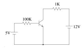
Figure 8: Transistor circuit (Example 2).
