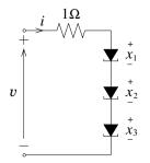
Figure 18: One-port tunnel diode circuit.
