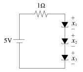
Figure 13: Three-tunnel diode circuit (Example 4).
