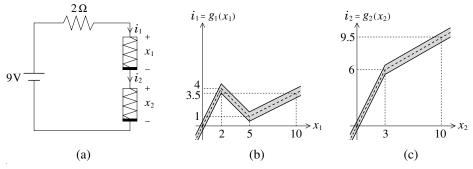
Figure 6: Circuit studied in Example 1 and the voltage-current characteristics of the PL resistors.
