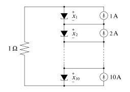
Figure 15: Ten-tunnel diode circuit (Example 5).
