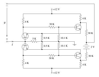
Figure 21: One-port transistor circuit.
